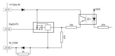
Figure 4-12 DigOUT3 Circuit – (analogously valid also for DigOUT4)
