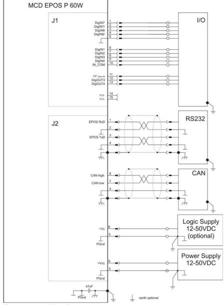
Figure 4-4 Wiring Diagram
