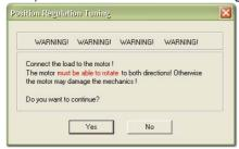
Figure 3-29 Confirmation of free running Shaft
